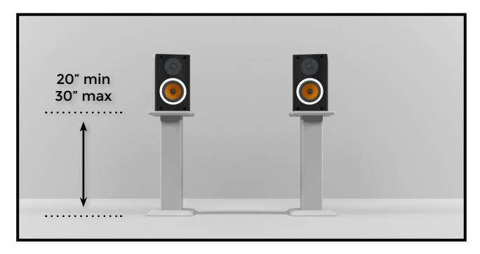
Use speaker stands or sit speakers on top of floating wall shelf or cabinet firmly secured due to weight of speakers.
